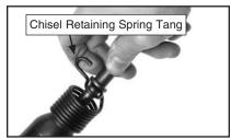
Figure 3. Chisel installation.
